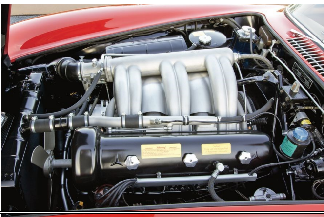
Mercedes-Benz 300 SL six-cylinder engine with mechanical fuel injection. Hemmings file photo.
