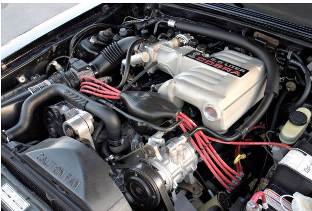
Ford 5.0L V-8 with multipoint electronic fuel injection. Hemmings file photo.
